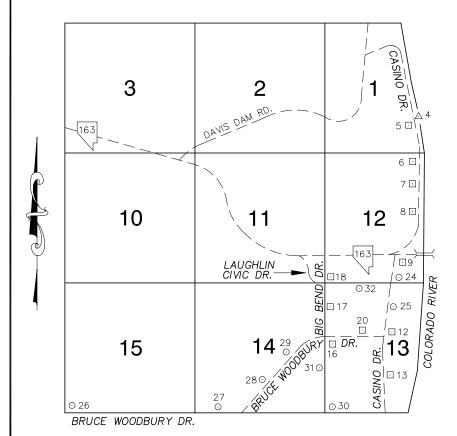
IN 1992, ELEVATIONS IN THE LAUGHLIN AREA WERE ADJUSTED TO NAVD 1988 FROM NGVD 1929 UTILIZING THE NATIONAL GEODETIC SURVEY'S VERTCON TRANSFORMATION PROGRAM VERSION 1.0. THIS PROGRAM HAS AN ESTIMATED ROOT MEAN SQUARE ERROR OF +/- 1 CM, AND A MAXIMUM ESTIMATED ERROR OF +/- 2.5 CM. THIS 2003 BENCHBOOK INCORPORATES THIS METHODOLOGY.
