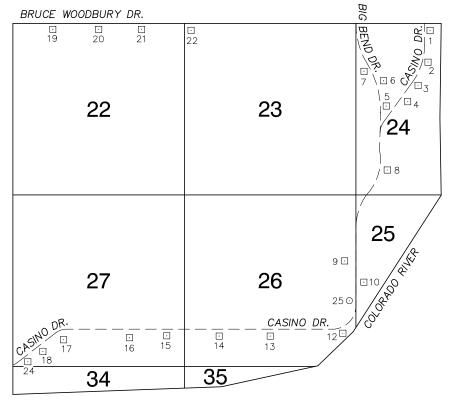
IN 1992, ELEVATIONS IN THE LAUGHLIN AREA WERE ADJUSTED TO NAVD 1988 FROM NGVD 1929 UTILIZING THE NATIONAL GEODETIC SURVEY'S VERTCON TRANSFORMATION PROGRAM VERSION 1.0. THIS PROGRAM HAS AN ESTIMATED ROOT MEAN SQUARE ERROR OF +/- 1 CM, AND A MAXIMUM ESTIMATED ERROR OF +/- 2.5 CM. THIS 2003 BENCHBOOK INCORPORATES THIS METHODOLOGY.
