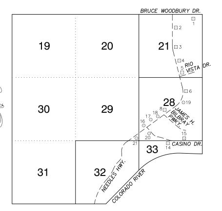
IN 1992, ELEVATIONS IN THE LAUGHLIN AREA WERE ADJUSTED TO NAVD 1988 FROM NGVD 1929 UTILIZING THE NATIONAL GEODETIC SURVEY'S VERTCON TRANSFORMATION PROGRAM VERSION 1.0. THIS PROGRAM HAS AN ESTIMATED ROOT MEAN SQUARE ERROR OF  $\pm$ 1 CM, AND A MAXIMUM ESTIMATED ERROR OF  $\pm$ 2.5 CM. THIS 2002 BENCHBOOK INCORPORATES THIS METHODOLOGY.
